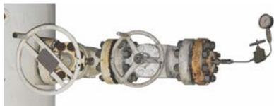
Typically, to monitor annulus pressure, a pressure gauge is installed on an instrument flange, with either 1 or 2 gate valves between it and the wellhead side outlet / annulus.
