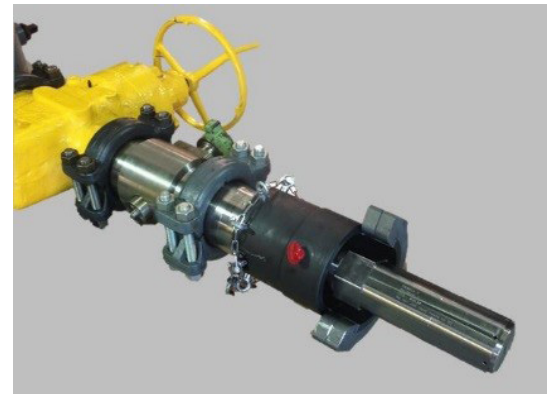
Figure 2| BB Lubricator during SIT with torque adapter
